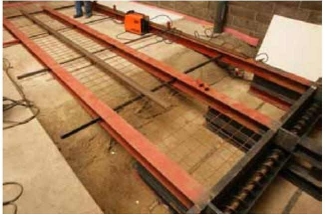
Bottom beams concreted to the floor. Pictured also cylinders, cylinder seals, rear wall elements and ready-fitted hydraulics. It is advisable to install these after the pusher rods and wall element.
