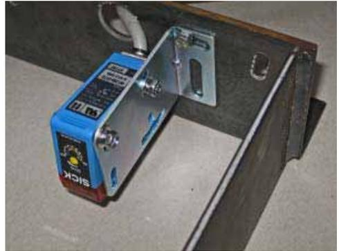
Adjust the identification distance with a screwdriver. Turning the adjusting screw anti-clockwise moves the indicator point on the upper scale clockwise. The identification distance is usually correct when the point is at 1 o'clock.
