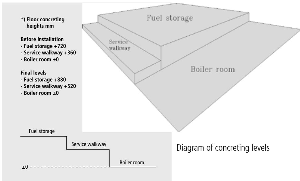
The concreting can also be done at the same time but then the supporting installation for the bottom beams must be ensured in some other way.
