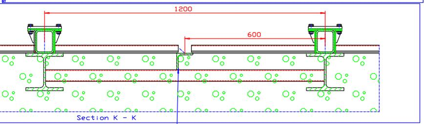
Welding supports are needed when using counter-pushers (recommended). The beam, e.g. L70, is not part of the delivery.
