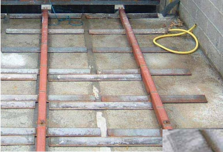
When the piston rods are in the inner position, place the control tunnels on top of the rods and fit them so that they are not in the path of the blades when the pusher rod moves backwards and forwards (300 mm). The distance between the upper edge of the pusher and the tunnel is about 10 mm.
