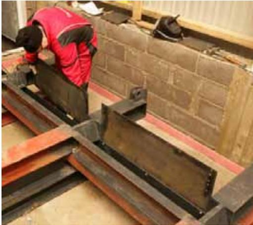
Before installing the stoker auger, fit the wall elements into position as you align them.
